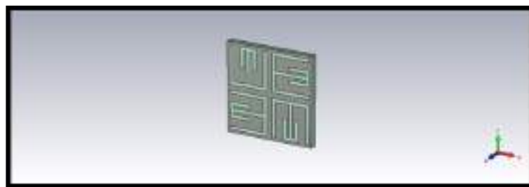
Figure 2: Schematic drawing of the proposed FSS (A) Periodic structure (B) Unit cell
