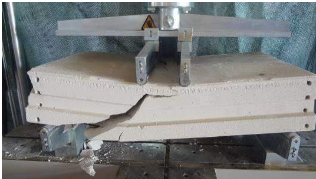
Figure 5 Failed RAACP (monotonic loading)
