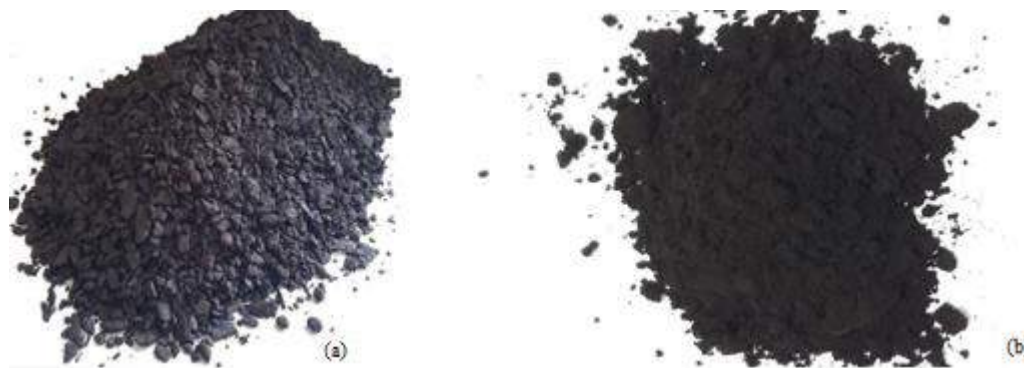
Figure 1. A Photographic View of Coal Particles Before (a) and After (b) Milling Process
