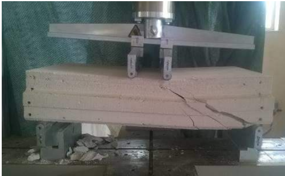
Figure 4 Failed RAACP (cyclic loading)
