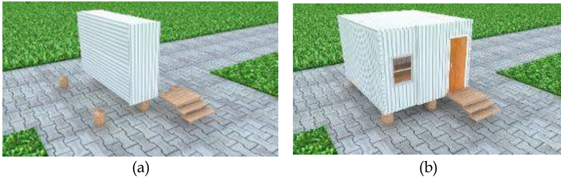
Figure 3 Winged shelter design (a) folded unit, (b) unfolded (after erected) unit
