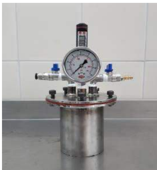
Figure 1. The Batch Reactor Used for Glycerol Ether Synthesis
