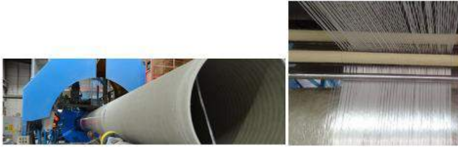
Figure 1. Continuous filament winding technique
